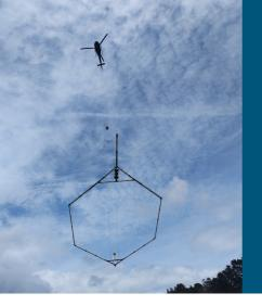
You may see a low-flying helicopter towing a large loop hanging from a cable during February and March. It will fly over the areas highlighted on the map and 'scan' down to about 300 metres deep underground, where we've never seen before. We won't be flying over towns or builtup areas.
